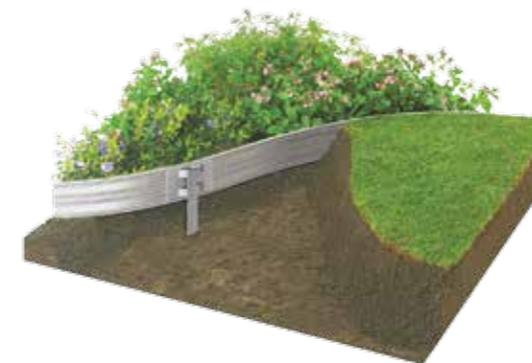
Standard installation method between two soft interfaces such as planting and lawn.
